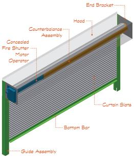
Auto-Set® Model CFS fire shutters can be designed to accommodate almost any opening variation. For a finished appearance when the housing is exposed McKEON offers a tubular concealed inboard motor option.
