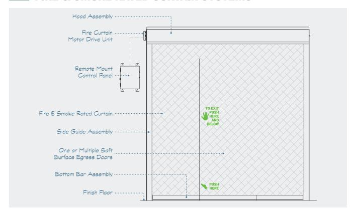
The McKEON D200E side guide configuration, with a maximum of a 1/2" reveal, can be surface or flush mounted making it virtually invisible in any application.
