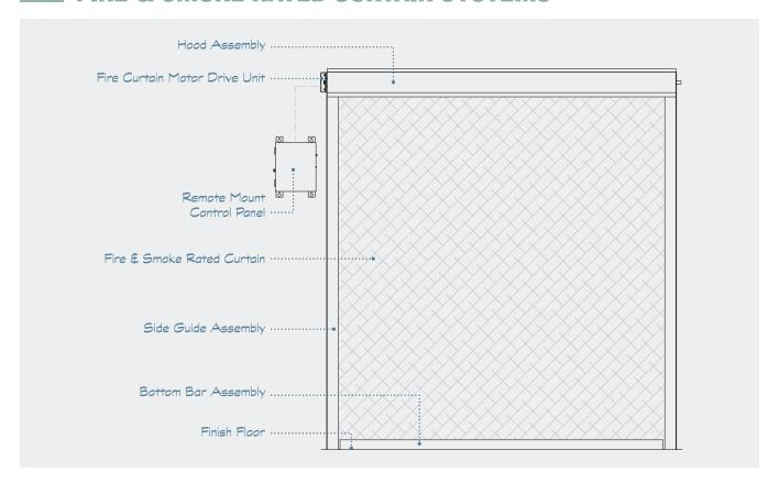
The McKEON D200 side guide configuration, with a maximum of a 3/8" reveal, can be surface or flush mounted making it virtually invisible in any application.
