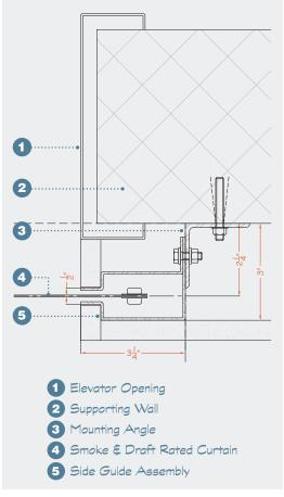
Side guides, with a nominal reveal, can be surface or jamb mounted making them virtually invisible in any application.
