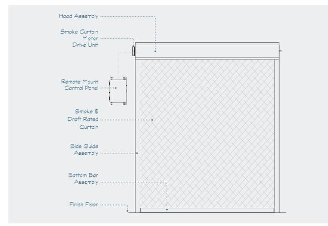
Side guides, with a nominal reveal, can be surface or jamb mounted making them virtually invisible in any application.
