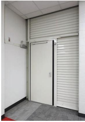
T2000 Series fire door assemblies incorporate either one or two deployable egress doors which are flush mounted in an adjacent wall. Upon activation by a building alarm or in an emergency condition, these complying egress doors swing into position. The doors then serve as side guides for the vertical coiling door assembly as it descends to provide complete protection from fire and smoke, and provide conventional egress as required.
