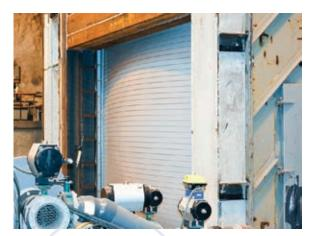
The SafeSpace 500 was subjected to both a positive and negative pressures equal to 1.2 times the 255 mph design wind load.
