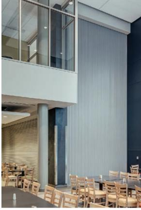
In this university application neither width nor height was a challenge for the \$4000 technology. Space, the primary concern, was easily conserved with this side coiling system which requires only a small boxed area for stacking rather than the deep-pocket storage space usually required. Notice also that the head track width is minimal and virtually invisible despite the extreme size of this 3-hour rated assembly.
