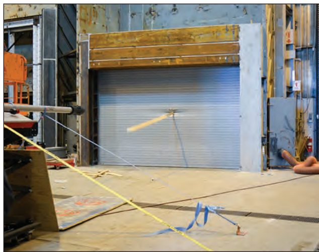
The SafeSpace 500 was subjected to both a positive and a negative wind load.
