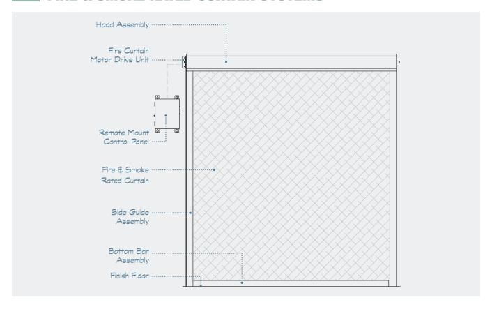
The McKEON D200 side guide configuration, with a maximum of a 3/8" reveal, can be surface or flush mounted making it virtually invisible in any application.
