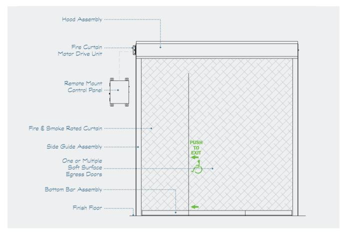
Side guides, with a nominal reveal, can be surface or jamb mounted making them virtually invisible in any application.
